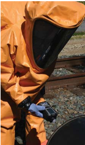
CBRN detection with the MultiRAE Pro
